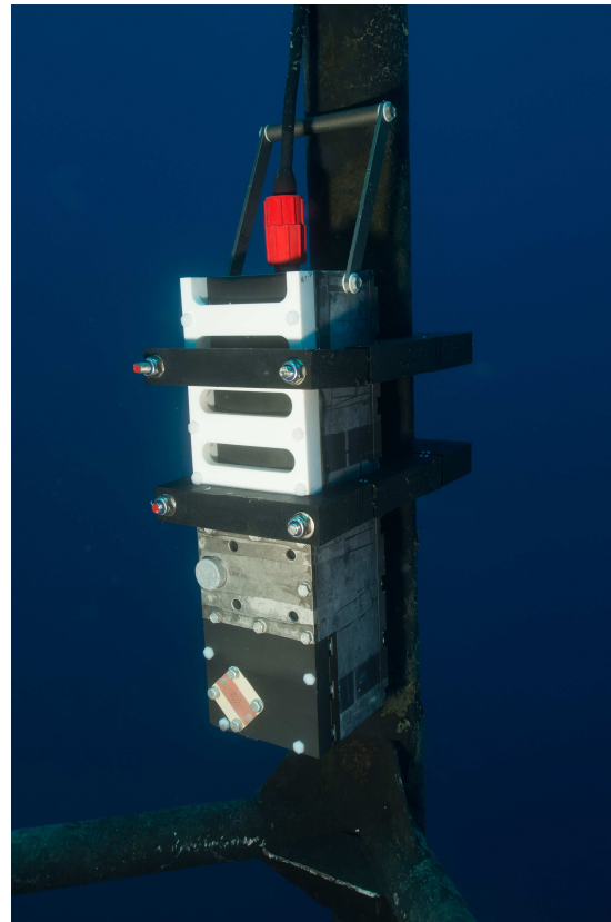
CTD plus optode (left) and pCO 2 CARIOCA sensor (right), as installed on the BOUSSOLE buoy at 10m depth (BIOCAREX project).
